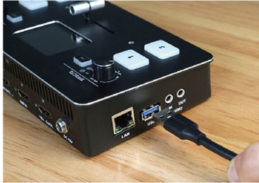
USB Output for Live Streaming with your Planet eStream Platform
